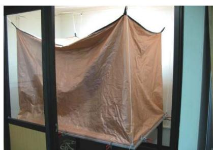
Fig. 6 Vibrating intrinsic reverberation chamber hanging on strings, picture extracted from Ref. [23]
