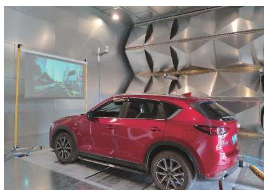
Fig. 9 Oscillating stirrer at the RC facility of Comtest Engineering, picture extracted from Ref. [29]
