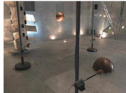
Fig. 18 Mechanical reverberation chamber with two hemispherical diffractors, picture extracted from Ref. [52]
