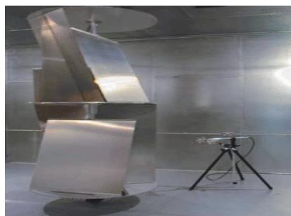
Fig. 4 Irregular reconfigurable stirrer in the RC at NPL,
